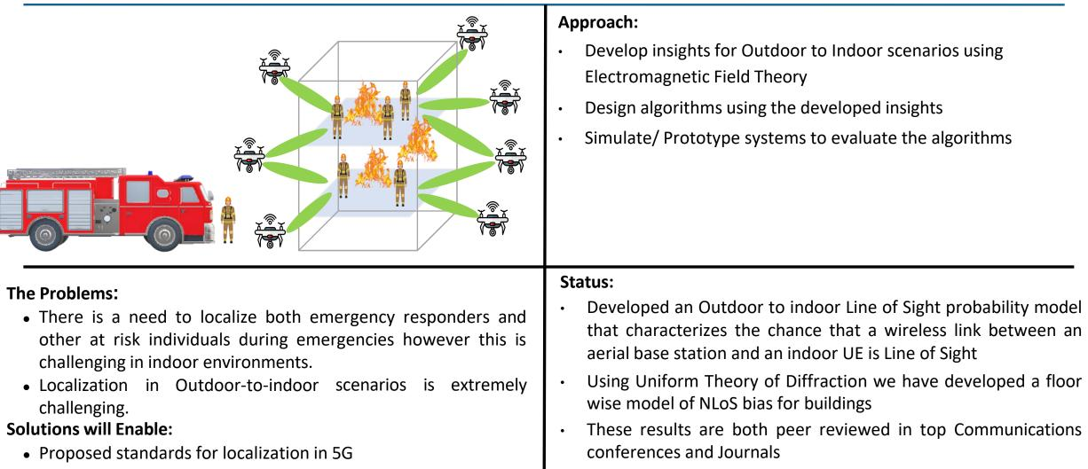
• Aerial UAV base stations can be employed to leverage advantageous locations outside buildings to obtain better signal propagation conditions
