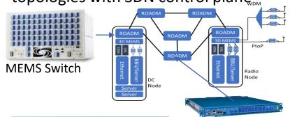
fast front-haul/midhaul/back-haul connectivity between radio nodes and edge cloud
