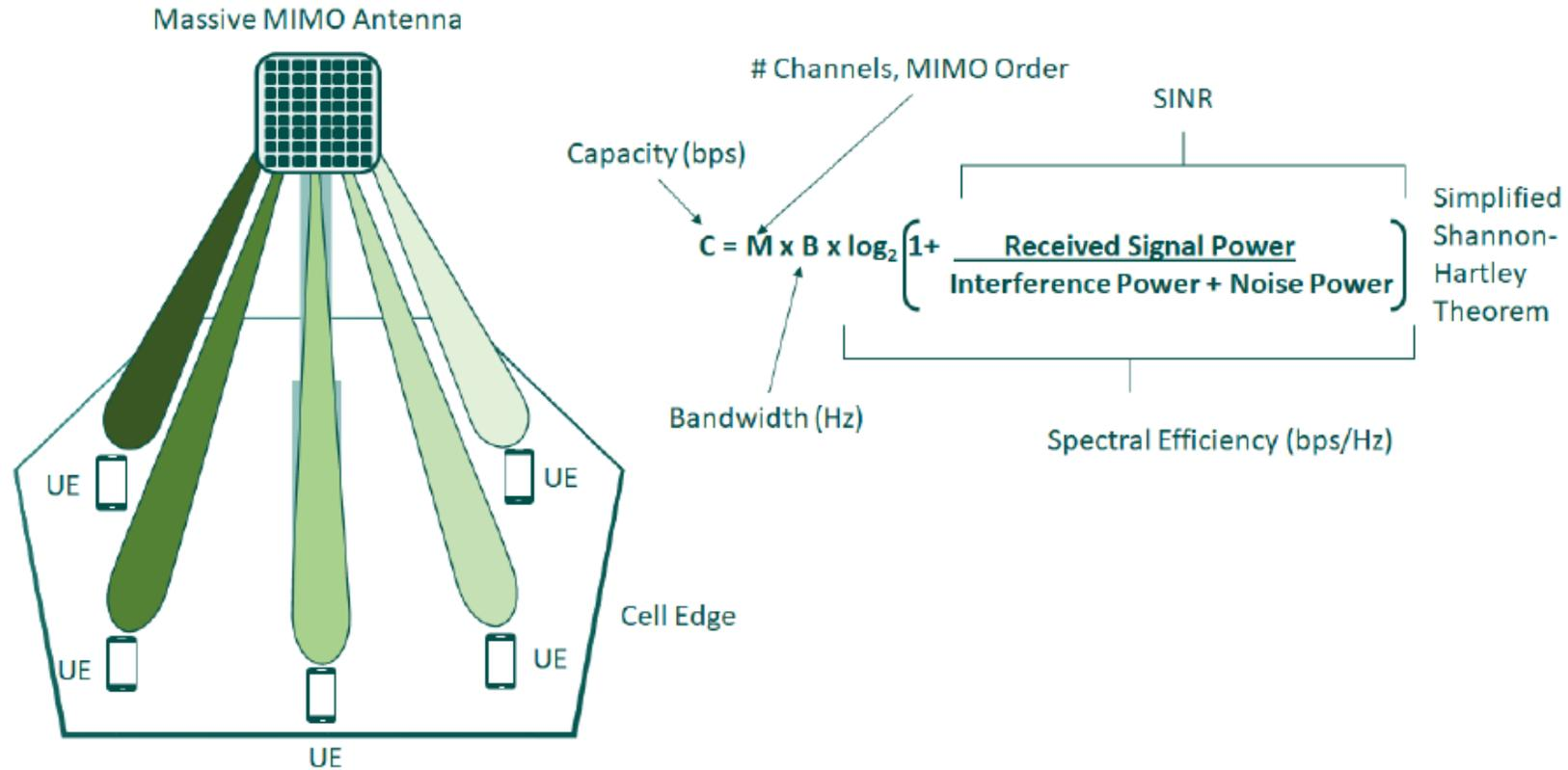
$$\text{Network Throughput (bps/km}^2\text{)} = \text{Cell Density (cell/km}^2\text{)} \times \text{Bandwidth (Hz)} \times \text{Spectral Efficiency (bps/Hz/Cell)}$$
